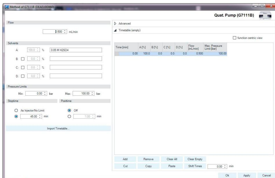
**Fig 3.** Quaternary Pump method parameters
