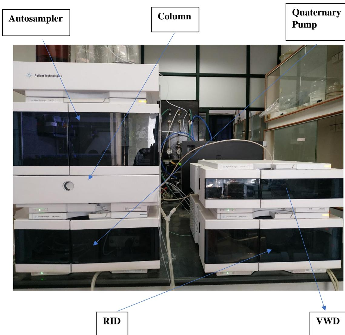
*Fig 1.* HPLC Instrument
